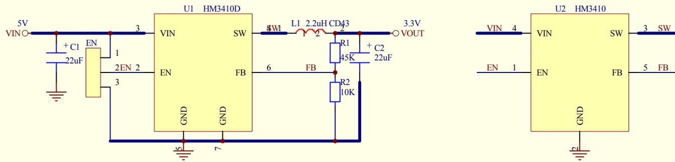
输出电压设置:  $V_{OUT} = 0.6V * (R1/R2 + 1)$
