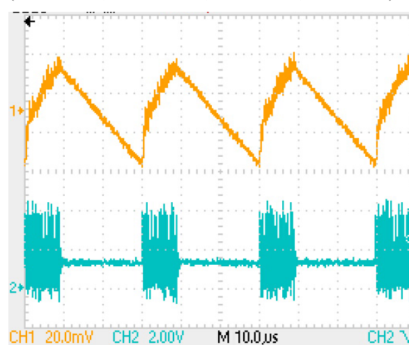
Buck Output Voltage Ripple Vs LX ( V_{BAT}=3.6V , I_{buck}=10mA , V_{buck}=1.2V , C_{out}=4.7\mu F )
