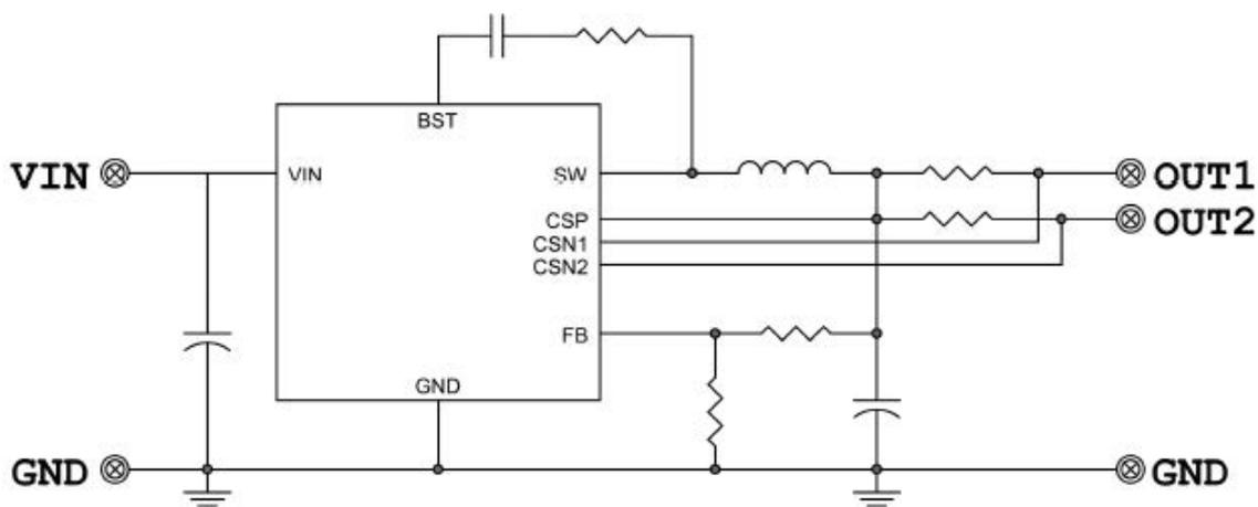
Note: When using a solid or ceramic input Cap, It is recommended to parallel a TVS diode.
