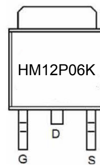
Marking and pin assignment
