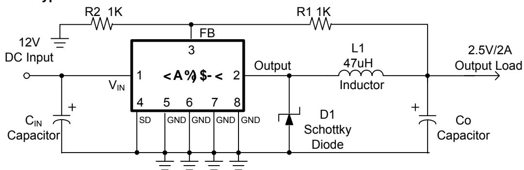
$$V_{OUT} = V_{FB} \times \left(1 + \frac{R_1}{R_2}\right)$$
