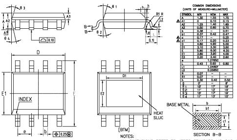
NOTES: SECTION B-B ALL DIMENSIONS REFER TO JEDEC STANDARD MS-012 AA DO NOT INCLUDE MOLD FLASH OR PROTRUSIONS.
